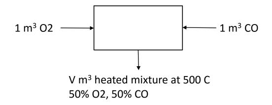
Observe that the masses of all streams can be multiplied by a common factor and the process remains balanced.
