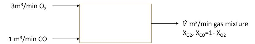
There are two unknown quantities ( $\dot{V}$  and X), so two equations are needed to calculate them Material balance equation for this nonreactive continuous process has the simple form input = output
